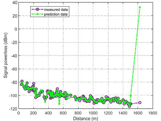
Fig. 8. Worst prediction result from training of 2- intermediate layers VNN with [36, 40] neurons
