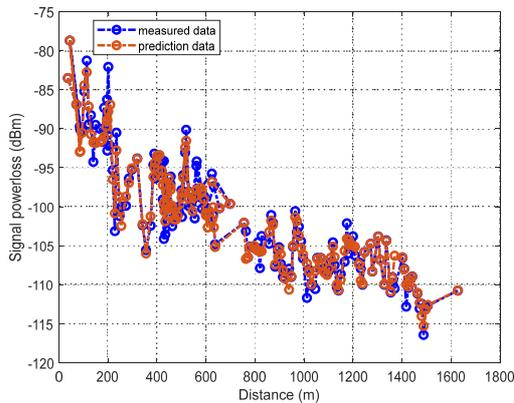
Fig. 4. Best prediction result from training of single intermediate layer VNN with 52 neurons
