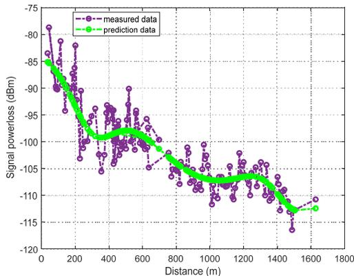
Fig. 5. First prediction result from training of 2- intermediate layers VNN with [4, 8] neurons
