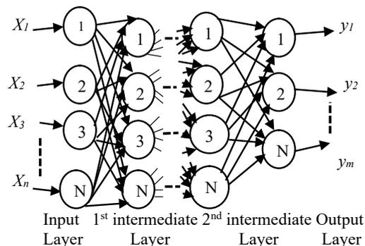
Fig. 1. Vanilla Neural Network with multiple intermediate layers (Adapted from V.C Ebhota et.al, 2018)
