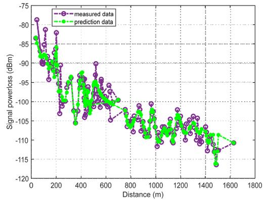
Fig. 6. Best prediction result from training of 2- intermediate layers VNN with [16, 20] neurons
