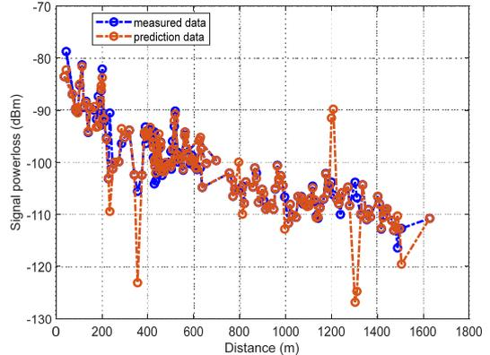
Fig. 7. Worst prediction result from training of single intermediate layers VNN with 80 neurons
