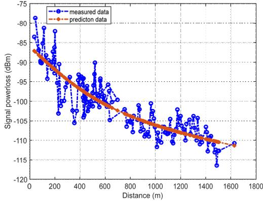
Fig. 3. First prediction result from training of single intermediate layer VNN with 4 neurons
