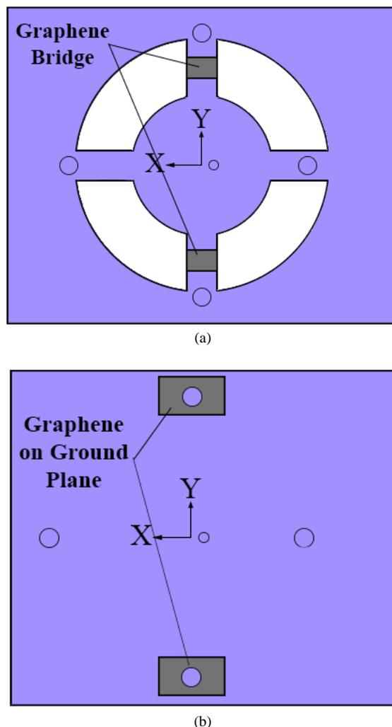
Figs. 9. Proposed solution for the graphene-based antenna: (a) top view; (b) bottom view
