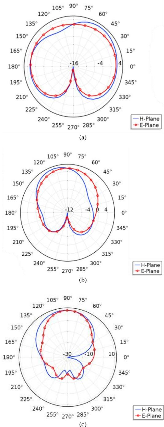
Figs. 7. 2D radiation pattern of the four-pin patch antenna computed at 2.43 GHz (a), 2.83 GHz (b) and 8.51 GHz (c). The beamwidth on the H-plane is about 170 degrees at 2.43 GHz, 75 degrees at 2.83 GHz and 55 degrees at 8.51 GHz
