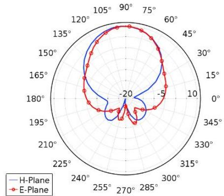
Fig. 3. 3D radiation pattern at 9.4 GHz computed for the three-pin patch antenna
