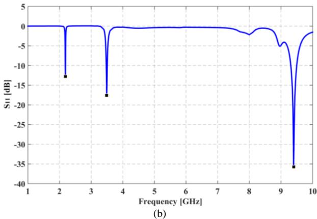
Figs. 1. Patch antenna with three shorting pins: (a) geometry. (b) Computed scattering parameter  $S_{11}$
