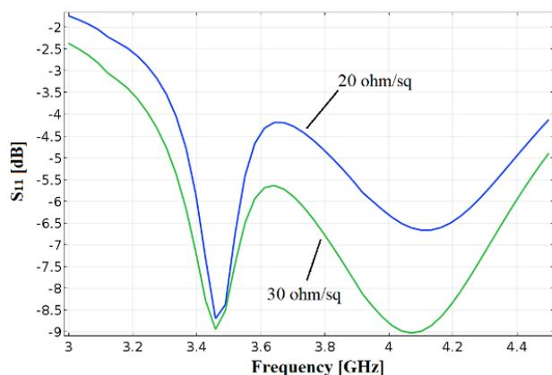
Fig. 11. Graphene-based antenna  $S_{11}$  parameter computed for 20 (blue curve) and 30  $\Omega/\text{sq}$  (green curve) sheet resistance
