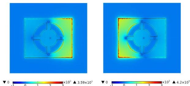
Fig. 6. Computed current density absolute magnitude ( $A/m^2$ ) of the four-pin patch antenna at 2.43 GHz (left image) and 2.83 GHz (right image)
