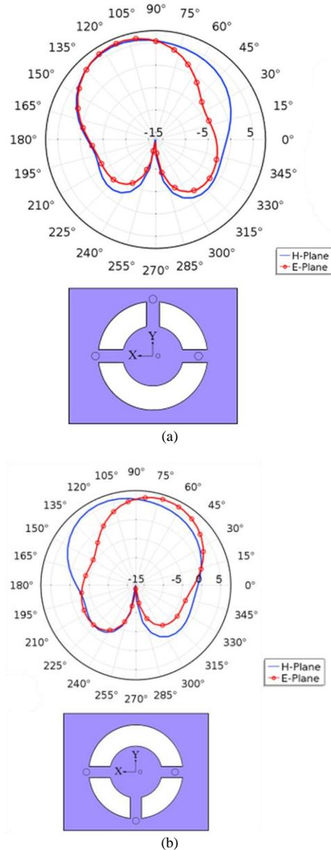
Figs. 2. Three-pin antenna radiation pattern computed at 3.5 GHz resonance frequency when the third pin position is at (a)  $Y > 0$  and at (b)  $Y < 0$
