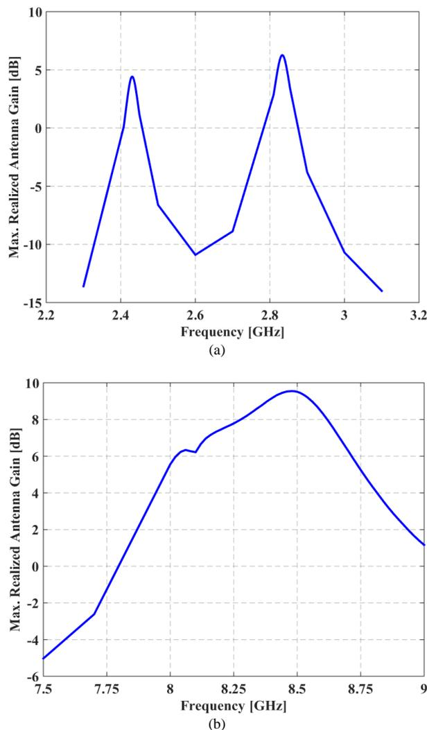
Figs. 8. Maximum realized antenna gain as function of lower frequencies (a) and higher frequencies (b) computed for the four-pin patch antenna
