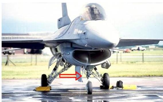
Fig. 1. Aircraft engine intake vortex at F-16 aircraft [10]
