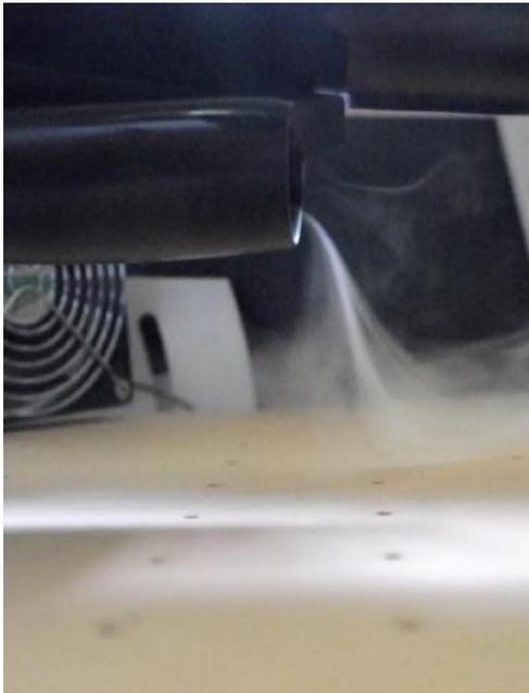
Fig. 2. Simulation of the intake system of fuselage turbine engine on the ground at a laboratory stand with visualization of the pathline [Photo A. Kozakiewicz]
