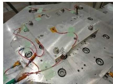
Fig. 7. The shock test's pickup sensors configuration for the solid-state-ceramic batteries mounted on the shock machine
