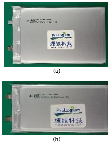
Figs. 1. Solid-state-ceramic battery ((a) LCB01, (b) LCB02) selected for evaluation test [15]
