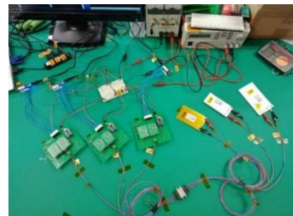
Fig. 6. Solid-state-ceramic battery charged and discharged before and after each test. Discharge condition: constant current (CC): DC: 0.5C, EOD: 2.8V. Charge condition: constant-current constant-voltage (CC/CV): CC: 0.5C, CV: 4.35V, LCB01 EOC: 97.5mA, LCB02 EOC: 72.5mA [15]
